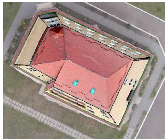
Fig. 4d. Texturing results in obtaining of a new image of a building at an orthophoto. Source: Own study.
