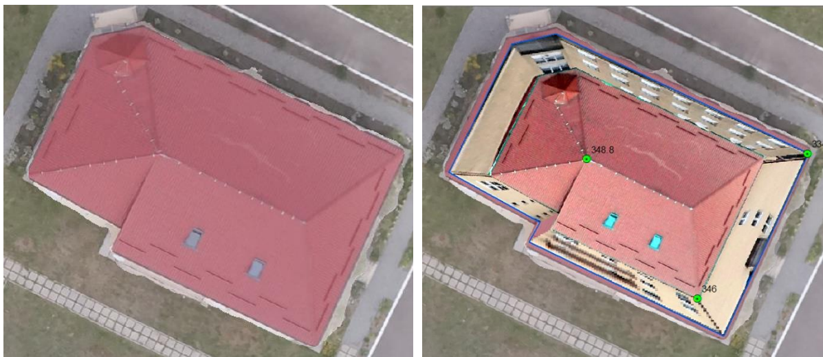
Fig. 6. Comparison of the two methods of formation of buildings images at an orthophoto: on the left – the traditional method, on the right – the proposed method. Source: Own study.
