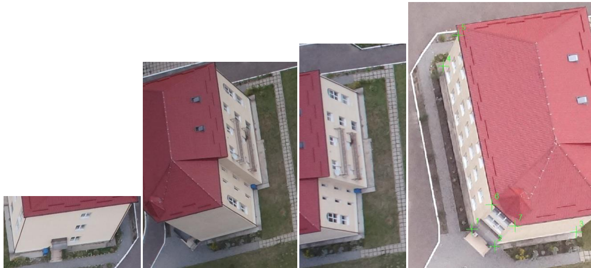
Fig. 5. Set of fragments of non-processed aerial images, selected for texturing of a wire-frame model of a building. Source: Own study.
