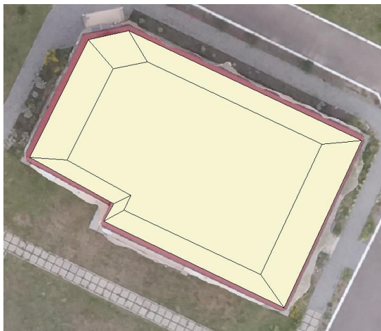
Fig. 4c. Results of projective transformation of representation of the top part of a building model. Formation of the grounds for walls texturing. Source: Own study.
