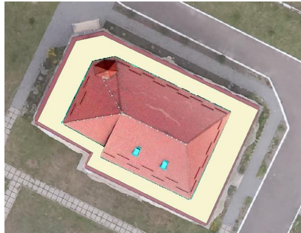
Fig. 4b. Results of projective transformation of roof representation. Source: Own study.
