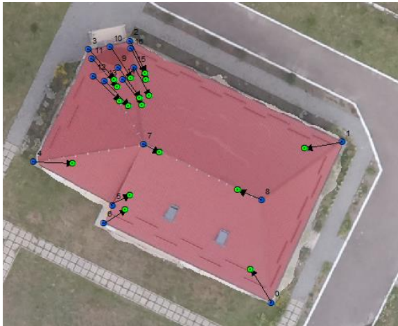
Fig. 4a. New positions of the points of a contour model of a roof, determined by the formulas 2, define essence of the projective transformation. Source: Own study.
