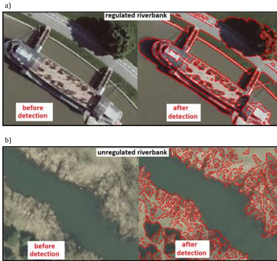
Fig. 4. Determination of the course of the shoreline using the Canny detection algorithm: (a) regulated riverbank (b) unregulated riverbank.
