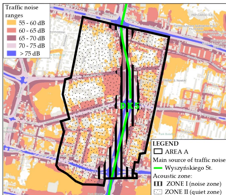
Fig. 3. The spatial range of acoustic zones with respect to the main sources on the ambient concentration road traffic noise imission map of the L_{DEN} indicator. Source: Own elaboration on the basis of (SZOPIŃSKA et al., 2017).
